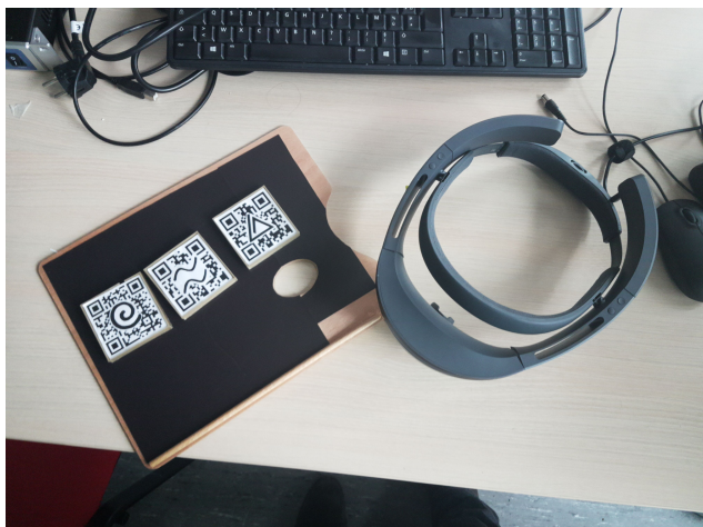
Figure 12: Closeup on the tangibles, the palette to use them on and the helmet. The AR Spells doesn't require much material wise.
